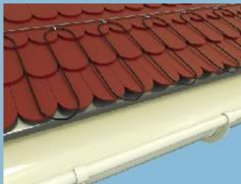
Example of heated roof edge
